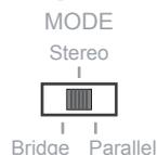
It is default configured in stereo mode (center position) whereby each amplifier channel is fed with an individual input signal. In bridge mode (left position), the power of both channels is merged for delivering double power to a single load. In parallel mode (right position), the inputs for channels 1+2 and channels 3+4 are linked, feeding the identical signal to both channels.
