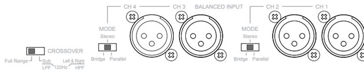
Each pair of input channels contains an operation mode switch, allowing switching the corresponding channels between stereo, bridge and parallel mode.
