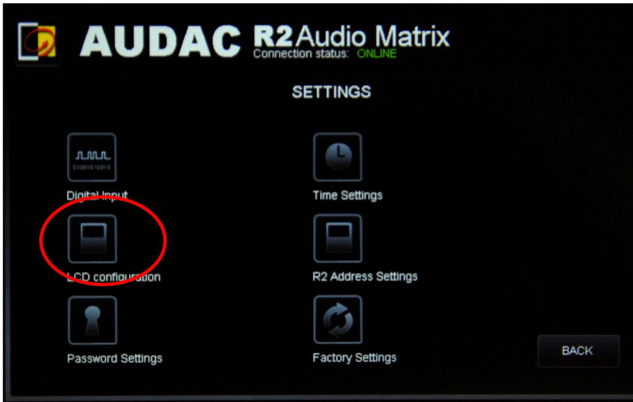
– At the LCD configuration screen, hold the “Update software” button for 3 seconds
