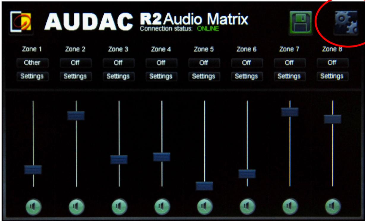
– At the settings screen, press the ‘LCD configuration’ button
