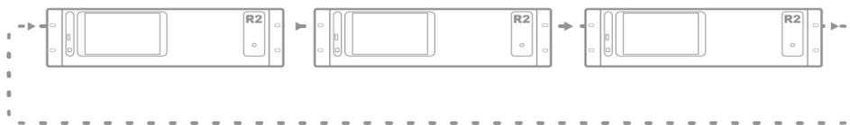
To control all the functions of all the R2's in one network, only one connection with the ethernet network of one R2 in the ring network is required. When multiple R2's are connected in a ring network, first a selection box will be displayed whereby can be selected which R2 you want to control.
