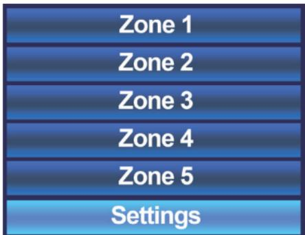
When returning back to the main menu, the latest selectable option is “Settings”. By selecting this option, changes to the settings of the wall panel can be made. After clicking this button, you will be redirected to the settings menu. The settings menu shows different options like: “Mic Phantom”, “Backlight”, “Screensaver” and “Info”.
