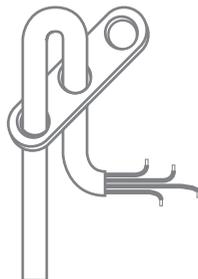
After the outer jacket is removed, the steel core needs to be terminated by a loop, making it possible to hang the steel cable core to the safety hook. The termination of the steel core should be done with the included screw cable clamp. Just insert the steel core through one side of it and return it through the other side. After this is done, tighten the screw from the cable clamp.
