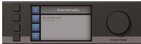
The functionality of the four tactile push buttons on the left side depends on the current mode and position in the menu structure. Icons on the left side of the display are indicating the current functionality linked with the buttons.
